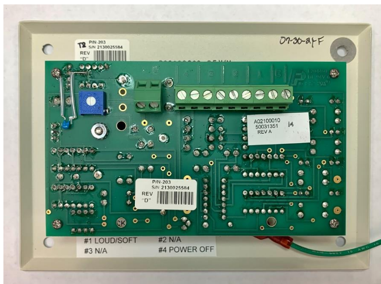
Figure 8-8 Back of 204 Nurse Station
